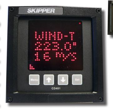
The SKIPPER CD401MR is a remote multirepeater for NMEA signals. It is designed for use with SKIPPER products together with products from other manufacturers, when these have an NMEA 0183 output.
